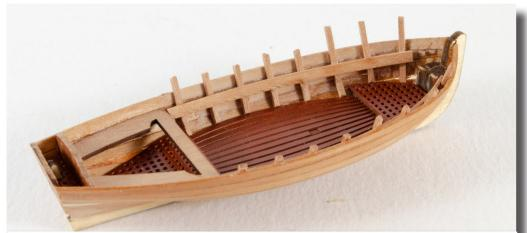
Now we need to fit the inside rail. I marked the top of the rail on my prototype as 2.5mm down from the top of the bulwark, but with evaluation, this would be better being located about 4mm from the top bulwark, but the sequence you see is the same. Split another 3mm strip and glue the rails 1.5mm wide, along the ribs using PVA and allow to set. Trim and sand the protruding ribs from the top of the bulwarks.
