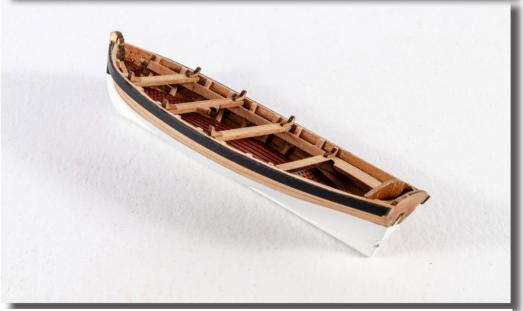
Add a strip of 1.5mm x 1mm wood along the top of the bulwark so it sits at the same height as bulwark top. Paint this black. Add the gunwale by simply cutting 1mm x 3mm wood strip to 1.5mm width, and gluing to the top edge of the bulwarks, leaving 1mm gaps for the oars to sit.
