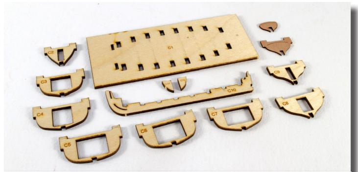
18ft Cutter, *optional feature:* Flirt would have been fitted with a cutter like this. First, we need to build a jig for creating the hull. Cut out all parts from the 2mm MDF sheet (C1 – C11) Also cut out C14 and C15 (bulkhead and stern board) from the 1mm wood sheet. Glue parts C2 – C15 into position on the Cutter Keel C10, and lightly apply glue to a couple of these bulkheads and slot the frame/jig into the Frame Base C1.
