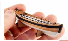
Drill a 0.8mm hole to accept the metal parts and glue using CA. Also drill a 0.8mm hole in the underside of the cradle parts and insert the sharp end of a brass pin so the cradle can be pinned to the deck.
