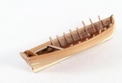
Using 3mm x 1mm strip, cut into either 1mm or 1.3mm widths, add the internal ribs, spaced roughly as you see in the illustration. You may want to soak the wood if it won't push into the internal contours.
